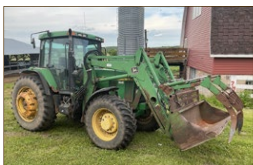
John Deere 7410 FWA with 740 Loader, 7' Grapple, triple hydraulic, 3-pt, 540/1000 PTO, PowrQuad Plus, left hand reverse, rear wheel weights, 18.4x38 tires (14.9x28 fronts)
