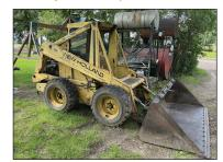
New Holland Skid Loader L775, SN 545488, Two Speed Gas WS Engine, Manual Quick Tach, 66" Bucket, 300 hours on new motor
