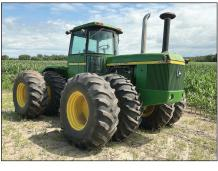
Rebuilt Transmission, Triple Hydraulic, 3-Pt., PTO, Quad Range, 23.1x30 Tires - insides less than a year old, SN 004640, shows 7432 hours, NICE condition
